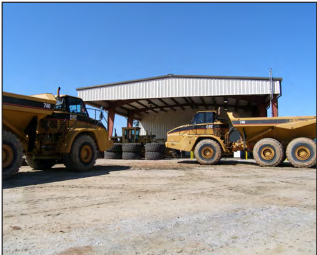
Off-Road Trucks Used To Hall Cover
